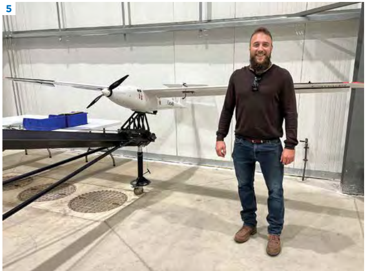
5. The fixed-wing drone is a development project that Taylor is currently working on. The goal is to monitor for forest fires (along with other surveillance applications). Currently, it can fly 24 hours at a time.
